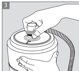
3 Open the front valve and remove the flexible pipe.
