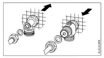
Fit the pipes with flat gaskets onto the twin nipples.
