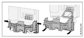
Press the two locking hooks and remove the lower part of the back panel towards the front.
