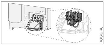
► Connect the power cable to the mains terminal (see chapter "Specification / Wiring diagram"). The specified voltage must match the mains voltage.
