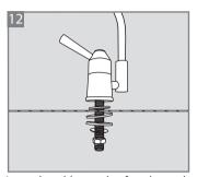
Insert the rubber washer from beneath the sink and fix the faucet in place.
