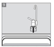
In case of wall-mounted installation of the faucet use the "L" connector to fix the faucet similar to the descriptions in picture 11-12.
