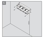
Select a proper place under the sink that has at least 25 cm (10") / 30 cm (13") from the floor to allow to insert the cartridges easily. Make holes into the wall to fix the filter adapter under the sink.
