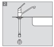
Detach the metal hose from the cold water supply under the sink.
