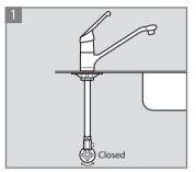
Lock the stop valve of the cold water supply line.
