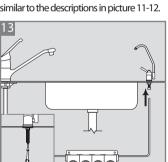
Connect the outlet tube with the drinking water faucet connector.
