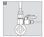
Open the diverter valve under the sink slowly. Check the whole system for water leakages.
