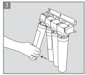
Pull the adapter connector to an angle of 45° while holding the filter.
