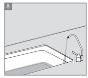
If there is no installation mistake or leakage keep the faucet open for 10 minutes to bring residual particles and air out of the unit.
