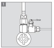
Close the diverter valve under the sink.
