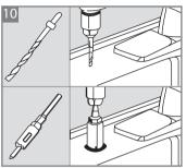
Select a proper place for the faucet. Drill a placement hole into the sink.
