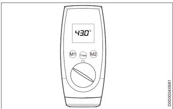
The temperature limit can be individually set between 30°C and 60°C
