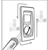
▶ In case of uneven surface, or installation of the wired control box is inside the shower room. The outer case should be glued together with the inner case. Finally, put the wired control panel inside.
