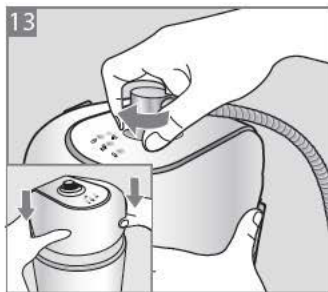
Put on the top cover and connect the flexible pipe to the nipple.
